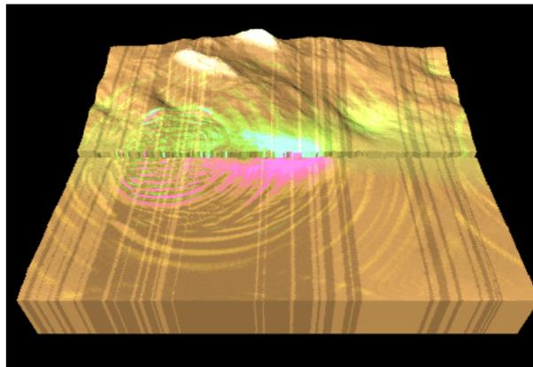
An earthquake simulated using a 2D particle-based Lattice Solid Model. Colours represent ground-velocity due to slip along a fault which bisects the model.
