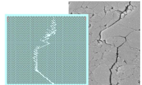
Dynamic failure of a brittle material using a model by the Laboratory of Nonlinear Mechanics. Crack patterns in the model are very similar to cracks in natural rocks.
